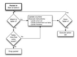
If a matching entry is found, the **instructions associated with the specific flow entry are executed**. If no match is found, the packet may be **forwarded** to the controller, **dropped**, or may continue to the **next flow table**.
