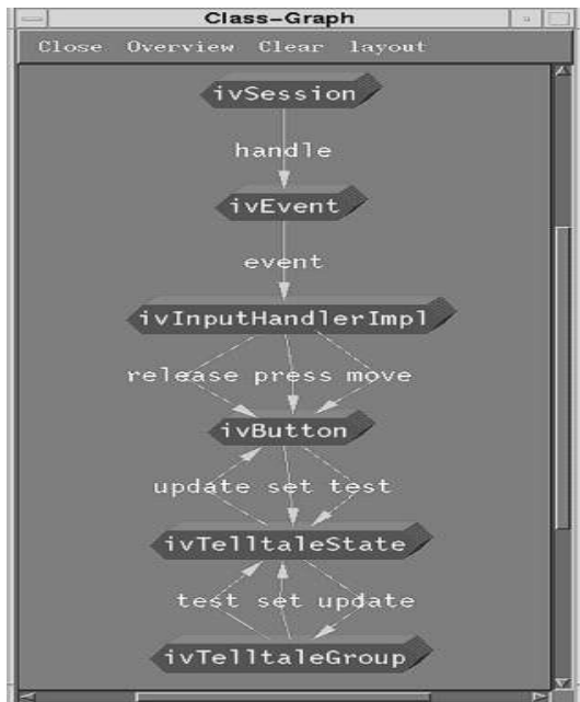
Figure 9: An example of the class graph. A class graph focuses on class interactions rather than object interactions
