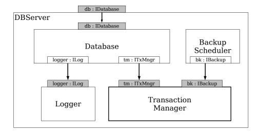
Fig. 1. Architecture of the DBServer component
