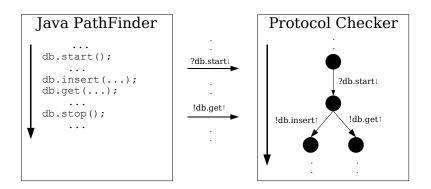
Fig. 2. Communication between the Java PathFinder and Protocol Checker
