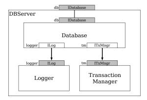
Figure 1: Architecture of the DBServer component
